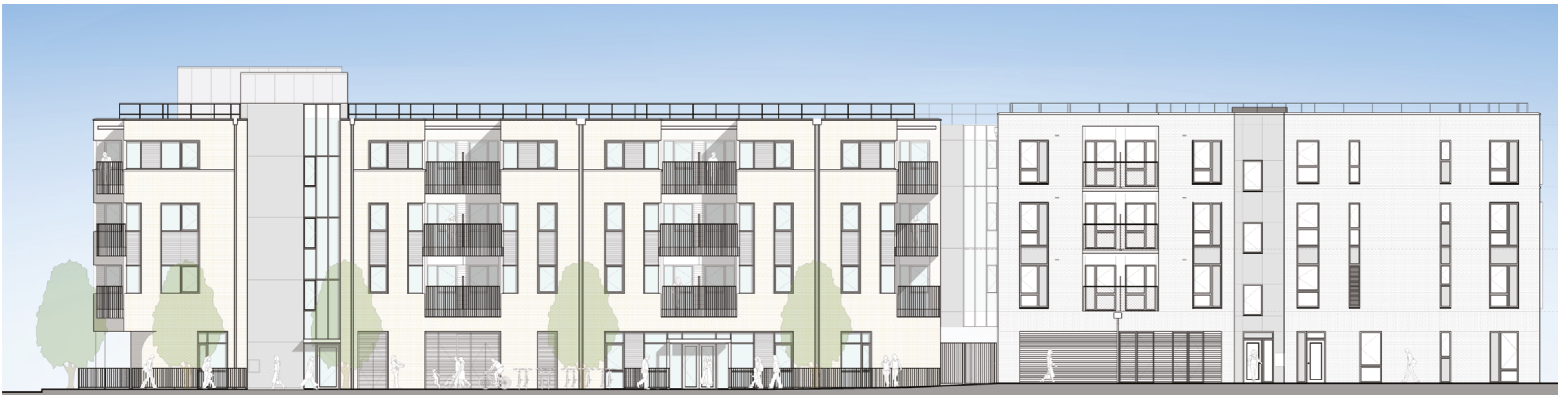
The proposed elevation to East Surrey Grove shows a building of similar proportions to Tayo Situ House but with the massing broken down into a rhythm of 'villas' incorporating a strong base floor, joined middle floors and with a horizontal emphasis for the top floor.
