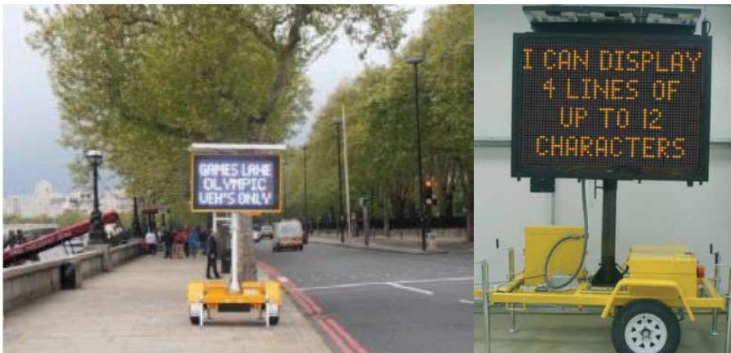
Figure 3-1 Variable Message Signs
