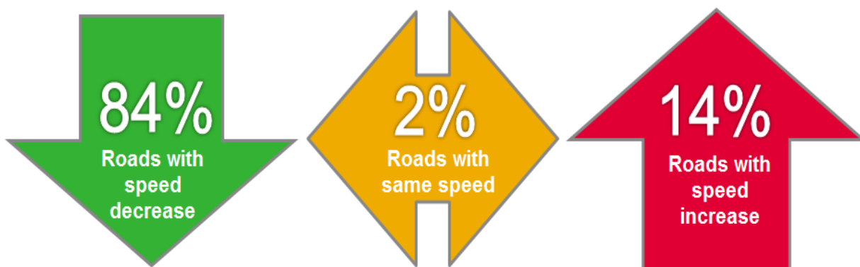
Figure 21. Percentage of roads in which speed decreased, increased or remained the same before and after the 20mph borough scheme (Source: Southwark Council Speed Surveys)
