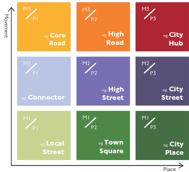
Figure 37. TfL Street Types Matrix based on Movement and function of the Place. TfL
