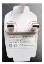
This charger does not comply - the pins are too close to the plug edge. It should not be on sale
