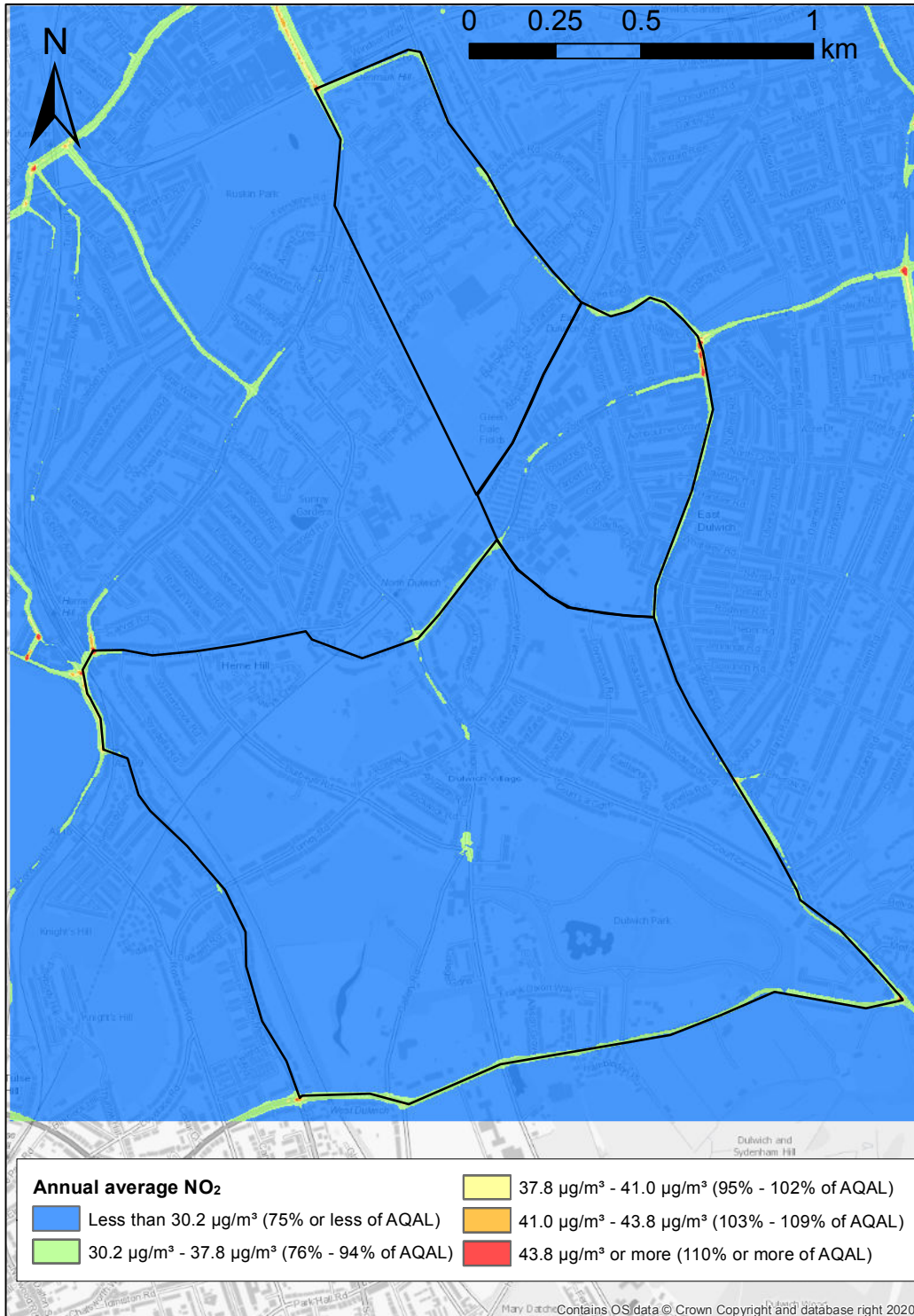
Figure 8.14: Post-scheme annual average NO 2 concentrations categorised by AQAL levels used in EPUK IAQM significance criteria calculations
