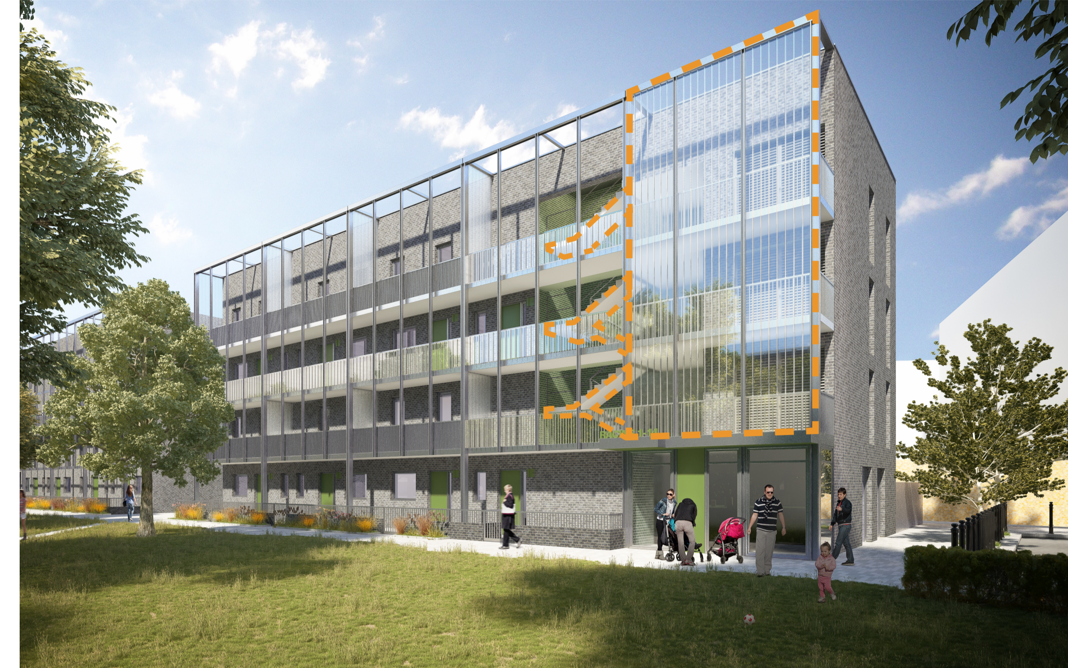
Racine: The visual above illustrates where the access stair was previously located towards the front of the Racine block. This has now been enclosed as indicated on the diagram below. The glazed aspect has also been omitted
