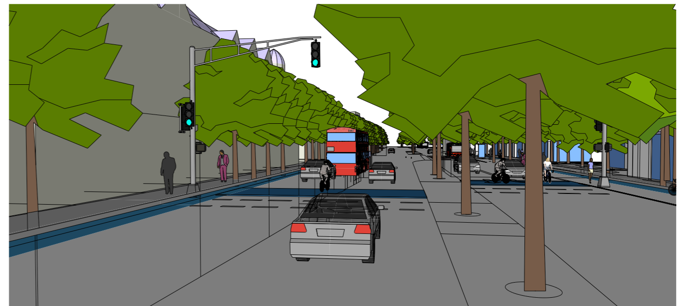
Indicative axonometric view looking towards Royal London Site, showing widened pavements, tree planting, segregated cycle lane and island bus stop
