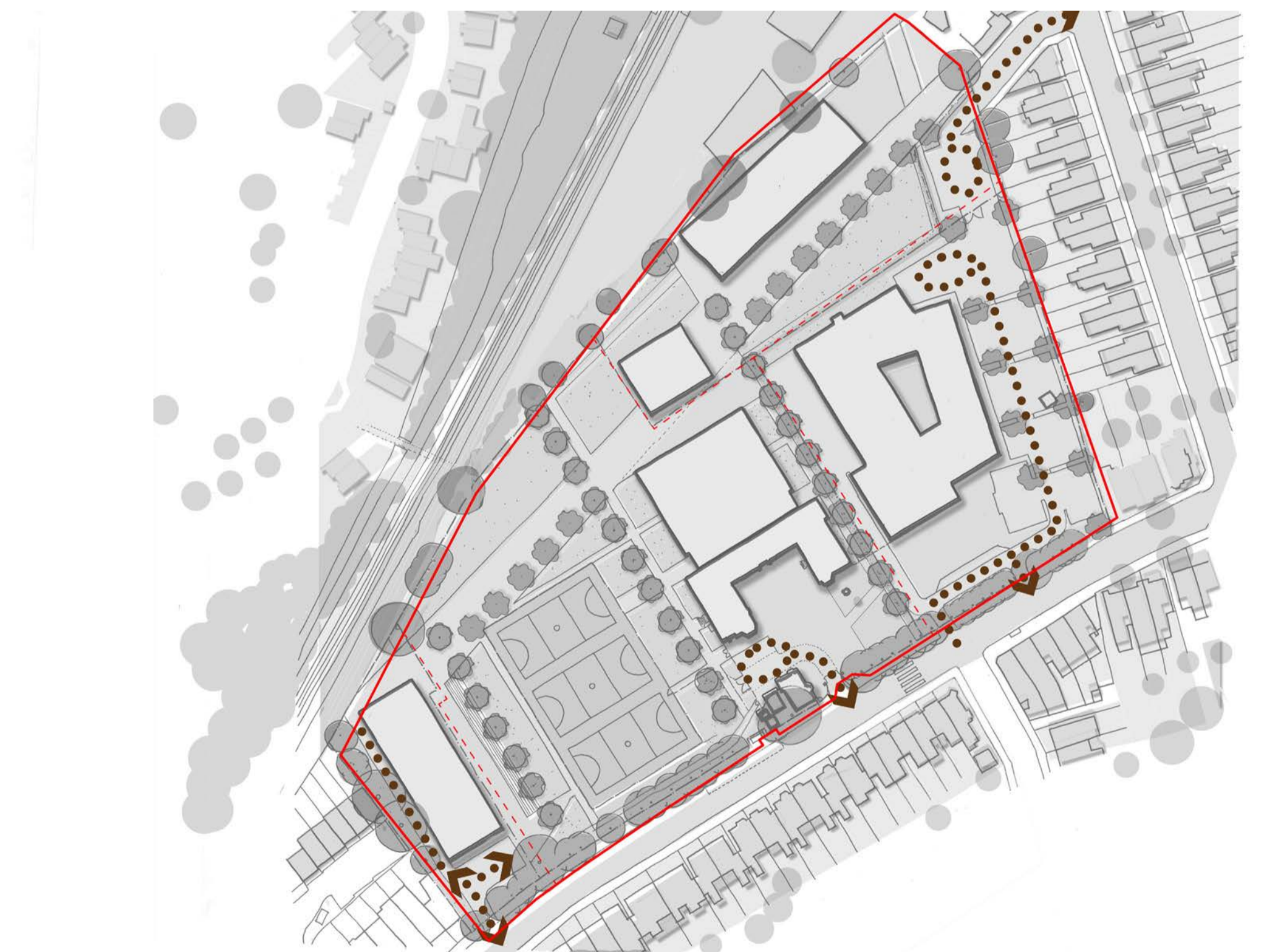
Service Vehicle Access
