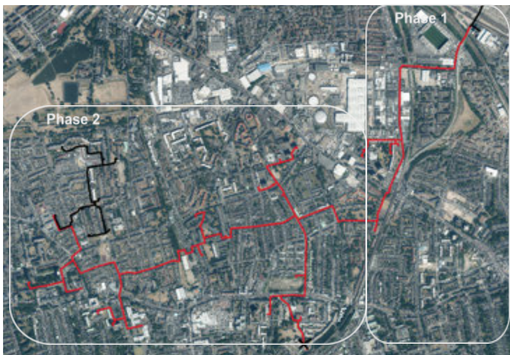
Figure 3. District Heating Network Expansion towards North Peckham
