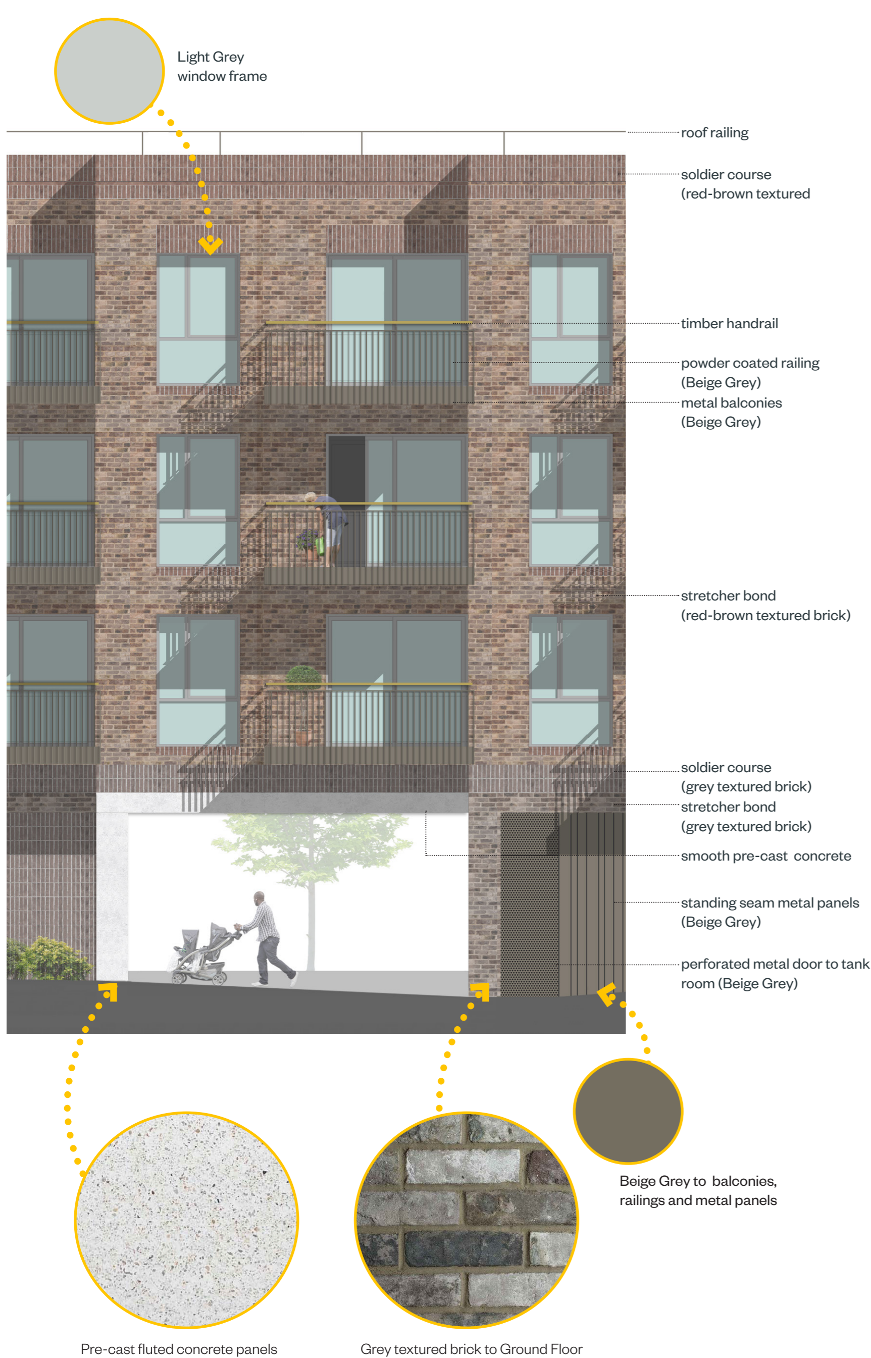
Proposed detail elevation - Street elevation
