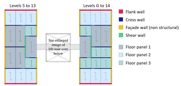
The residential towers are constructed with one-way spanning floors that span between cross walls and flank walls. On the long faces the façade panels are non-structural. Lateral stability against wind loading on the broad face is provided by the cross and flank walls. Lateral stability against wind loading on the narrow face is provided by the single shear wall.
