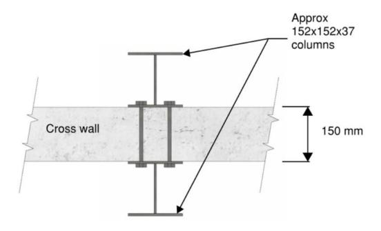
8. Cross wall/floor cross wall junction cross walls separating 1 and 3 bedroom flats (Floors G to 4) – Add steel beams.
