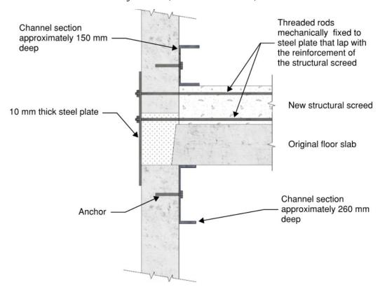
6. Typical flank wall to floor joint walls (Floors G to 7) – Add mechanical connections to connect flank wall back to floor diaphragm.
