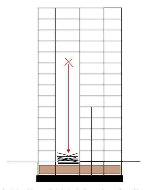
Further the loss of floors could also lead to the disproportionate collapse of the structural walls as the loss of horizontal restraint would mean that the walls would buckle. Hence the floors cannot be allowed to fail.
