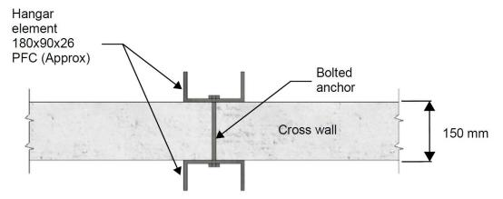
2. Typical Flank walls (floors 8 and above) – Add steel hangers
