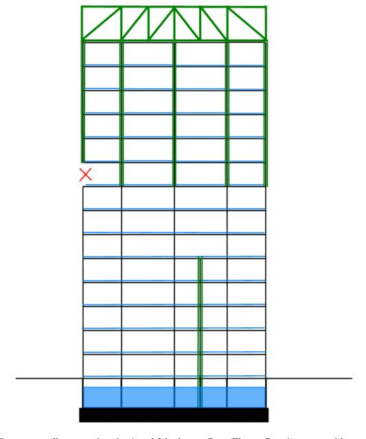
The cross walls separating the 1 and 3 bedroom flats (Floors G to 4) are not able to withstand 17 kPa by arching as they have no load from the floors above. As such it is proposed to install steel columns and beams designed to act as key elements to withstand 17 kPa to create an alternate load paths in the event of loss of this cross wall (see image below).
