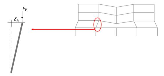
Further, the loss of one wall (in the manner shown above) would shed more load onto the adjacent walls. These loads would be further amplified due to the dynamic nature of a sudden wall loss due to an accidental event such as a gas explosion. The connections and elements at Ledbury Estate would not be able to accommodate these large forces.
