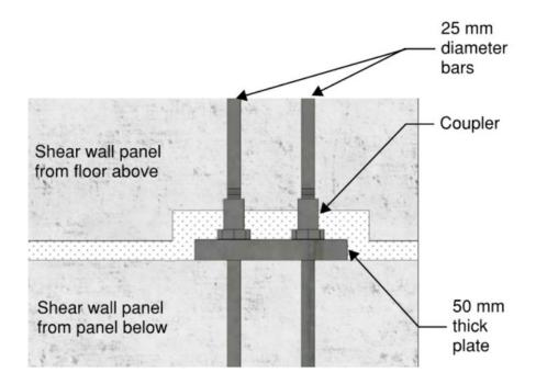
The connections in Large Panel Systems are known to be vulnerable to the quality of the site workmanship. Evidence of poor site workmanship was found during the investigations with sand instead of grout found in one of the wall to wall connections.
