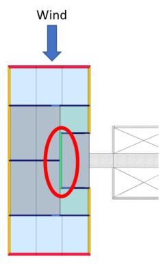
Since this wall is very lightly reinforced (as shown in Section 2.1.2) it is susceptible to "second order" effects. Calculations show that this shear wall is just strong enough to resist modern wind loads.
